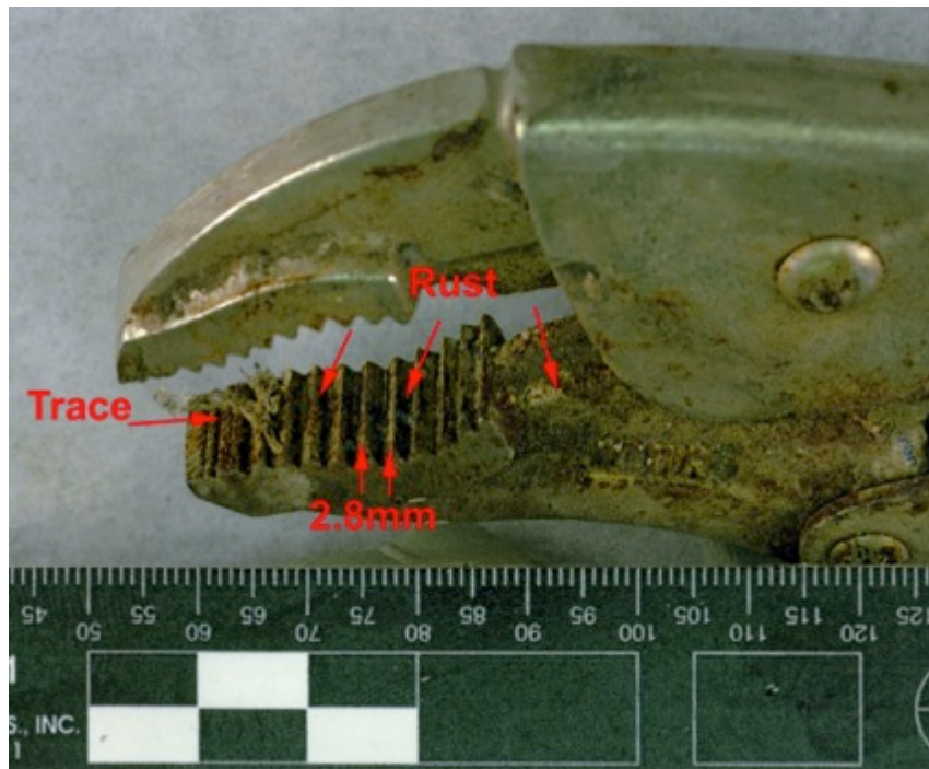
Photo 1-4 Vise grip with undisturbed traces of old twine and serrated teeth with undisturbed deposits of rust on lower jaw.
