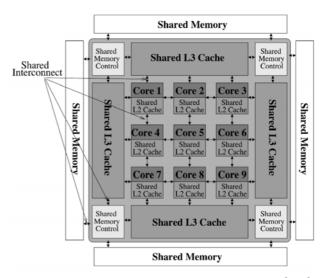
Fig. 8 A typical multicore system. Reproduced from [130].
