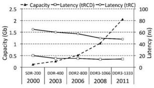
Fig. 3 DRAM Capacity & Latency Over Time. Reproduced from [106].
