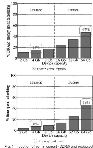
Fig. 1 Impact of refresh in current (DDR3) and projected DRAM devices. Reproduced from [111].
