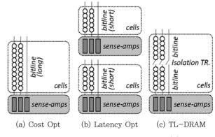
Fig. 4 Cost Optimized Commodity DRAM (a), Latency Optimized DRAM (b), Tiered-Latency DRAM (c). Reproduced from [106].
