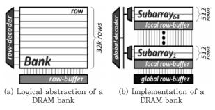
Fig. 2 DRAM Bank Organization and Subarrays in a Bank. Reproduced from [92].
